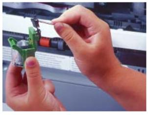
10. Slide the ink cartridge carrier into the desired position.
